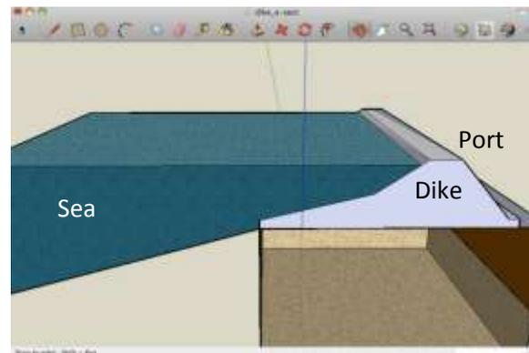
Figure 1. Typical Credible Minimum-criteria Dike Design.
